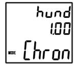
*Chron* mode has a resolution of a 1/Hundredth of a second. This is the standard mode used for the majority of timing applications.
