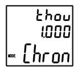
1/Thousandth mode is similar to the *Chron* mode but displays 1/1000th of a second resolution. In this mode the display will only time to 9.999 seconds. This mode is useful in timing short spans between the start and finish where extra resolution is needed for differentiation. All of the functions work the same as the "Chron" mode.
