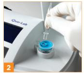
When prompted press reagent bead into cartridge using the reverse end of the sampling tool.
