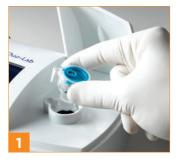
Scan lot calibration barcode. Remove foil from cartridge and insert into analyzer.
