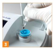
Insert sample tool into cartridge and snap off handle.
