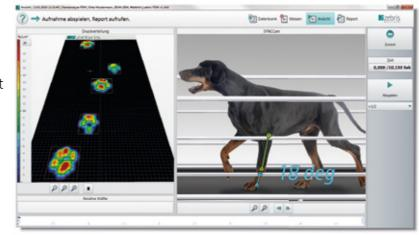
equipped with a calibrated pressure sensor matrix and one or several synchronised cameras.
