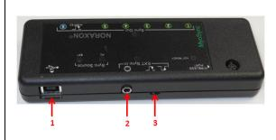
1 USB Port – A to B style to USB connection 2 External Sync Port – Sync in allows the MyoSync to accept a sync signal from another source and time 3 Invert Signal – Inverts or does not invert the sync signal depending on the direction of the switch
